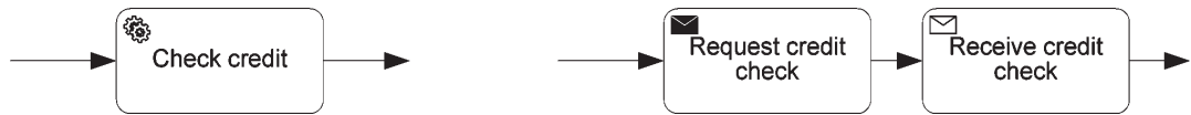
Figure 7-17. Use Send and Receive tasks for long-running services, Service task for short-running
