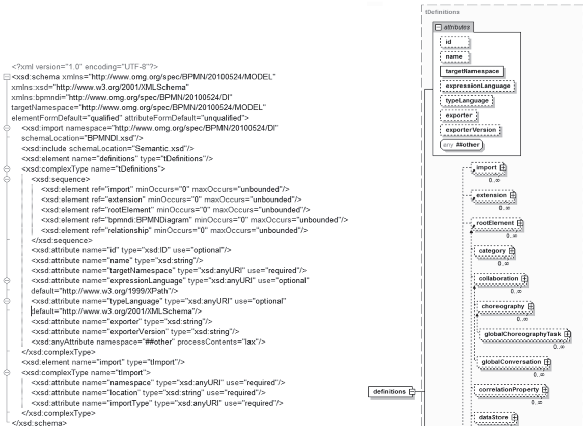
Figure 12-2. Text and Graphical views of the BPMN schema in XML Spy
